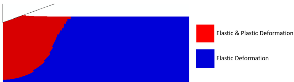
Fig. 3. The actively yielding elements (AC_Yield output) from ABAQUS used to estimate the volume of the plastic zone under the indenter during nanoindentation experiments. The red elements represent the elements undergoing plastic deformation, while the blue elements undergo elastic deformation only (For interpretation of the references to color in this figure legend, the reader is referred to the web version of this article).
