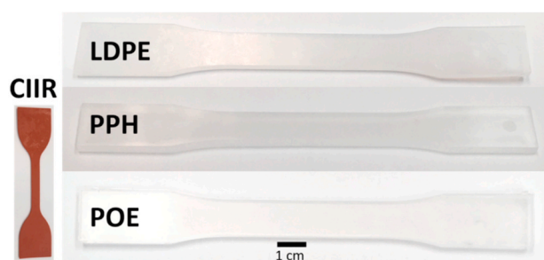
Fig. 2. Tensile specimens of the polymers investigated. CIIR-chlorobutyl rubber, LDPE-low-density polyethylene, PPH-polypropylene homopolymer, POE-polyolefin elastomer.
