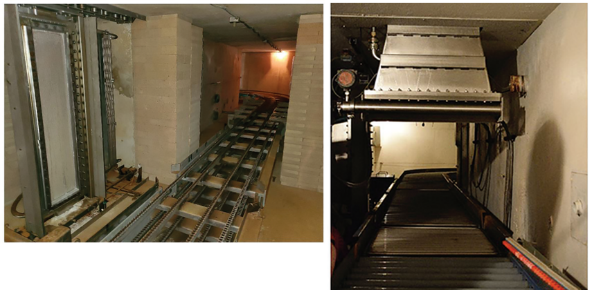
Figure 1: Examples of X-ray and electron-beam installations; scan horns are present in both installations. SOURCES: STERI-TEK (LEFT) AND TEXAS A&M UNIVERSITY (RIGHT)
